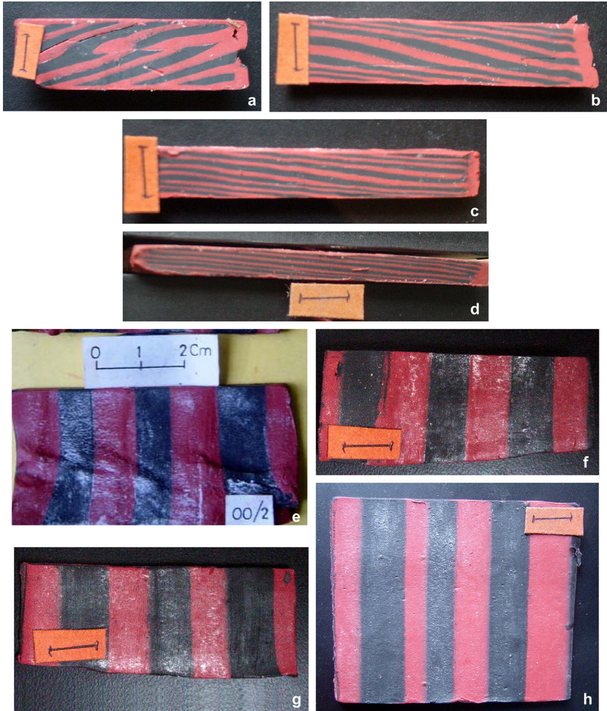
Fig. 6. (a–d) ABCD face of the deformed model after 50%, 65%, 78% and 125% of strain. (e–h) The corresponding ADPQ faces at different stages of deformation. Initial \theta was 30^\circ . Scale bar 1 cm. Note that from initial to final stage of deformations, \theta is greatly reduced but the average width of the stripes has not changed much.
